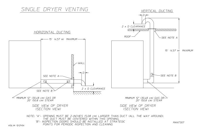
**IMPORTANT:** For extended ductwork runs, the cross section area of the ductwork can only be increased to an extent. Maximum proportional ductwork runs **cannot** exceed 15 feet (4.57 meters) more than the original limitations of 15 feet (4.57 meters) with three (3) elbows. When the ductwork approaches the maximum limits as noted in this manual, a professional heating, ventilating, and air-conditioning (HVAC) firm **should be** consulted for proper venting information.
